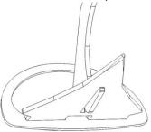
3 – Next, carry out the subsequent coupling of the roll plate (3) to the fluke (2) as sown:
