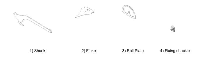
**2** – Take hold of the shank (1), placing it near the fluke (2) and insert the hook-shaped protruding into the central rectangular hole of the fluke obtaining a position of both pieces as shown figure:
